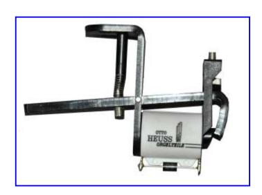
The action magnet armature can be adjusted by a spring. This makes it possible to optimise the magnet's tensile force. The limiter above the armature is easily accessible. This includes deviant to works settings if needed. The magnet is to be adjusted exactly to the windchest and then later fine adjusted.
