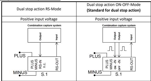
The RS-OUT is an output for the combination capture system, it shows if the stop is activated.
