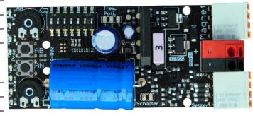
If dip switch 5 is switched on, the LEDs of the inputs Setzer-AN [setter-on] and Setzer-AB [setter-off] light up inverted to normal operation. (Similar to input "Funktion" [Function])
