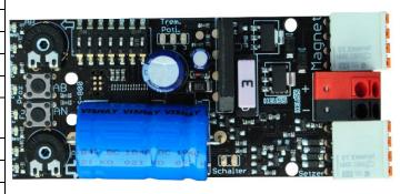
If dip switch 5 is switched on, the LEDs of the inputs Setzer-AN [setter-on] and Setzer-AB [setter-off] light up inverted to normal operation. (Similar to input "Funktion" [Function])
