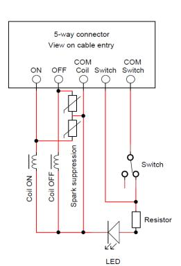
The reed contact is specified for 250mA. However, induction voltage (sparks) can also damage the reed contact. Provide sufficient spark suppression at the magnet to be switched. If this is not sufficient, an amplifier circuit or similar is necessary to protect the contact from sticking. No capacitive loads (capacitors) may be switched.
