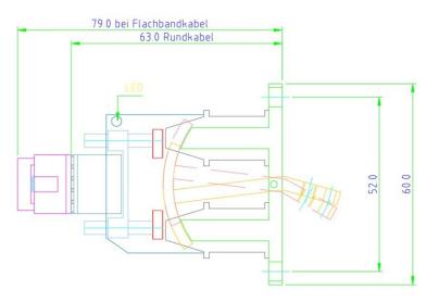
(Usually connected via round cable, resulting in a total length of 63 mm)
