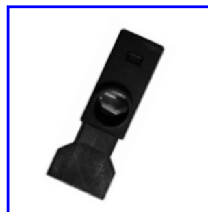
4265-104 Supply plug - Insulating plastic - 125 A - Lift terminal - Rigid wire 10 mm 2 - 25 mm 2 - Litz wire 10 mm 2 - 16 mm 2
