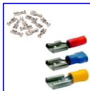
Flat plug sleeves for cable 4265-105 2.8 mm wide for 25 to 22 AWG 4265-106 2.8 mm wide for 20 to 17 AWG 4265-107 6.3 mm wide for 15 to 13 AWG 4265-108 6.3 mm wide for 11 to 9 AWG Our wire flat plug pliers 6060-031 are just right for our wire flat plug sleeves 20 to 9 AWG.
